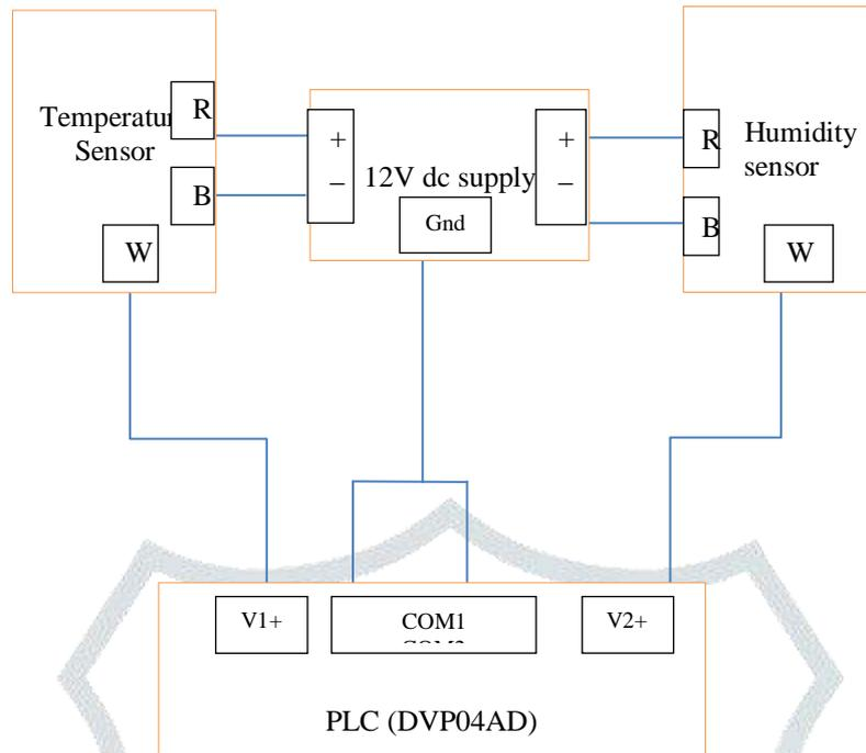
Fig 4: sensors connections to PLC with power module of 12Vdc.
