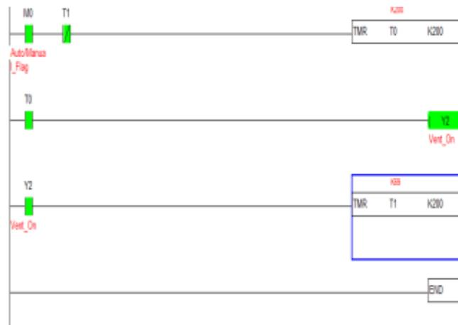
Fig 8: Ladder diagram for lighting system.
