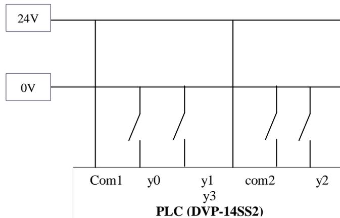
Fig 3: PLC output module electrical circuit.
