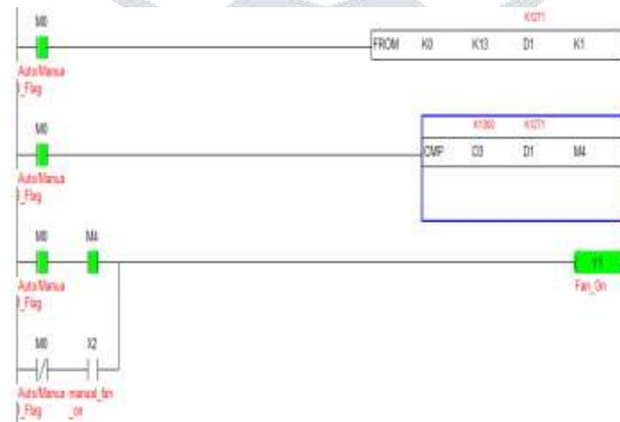
Fig 7: Ladder diagram for temperature control system.
