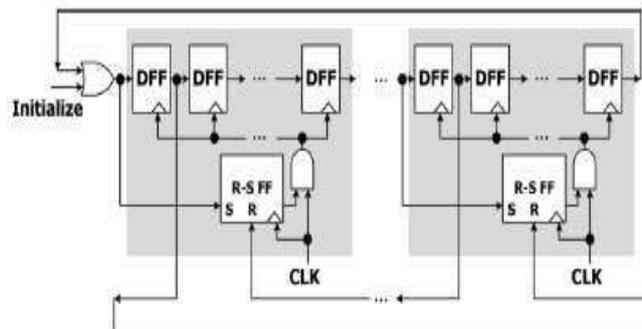
Figure 3 Ring counter with RS flip-flop
