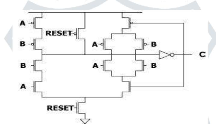
Figure 4 Logic Circuit of C-element
