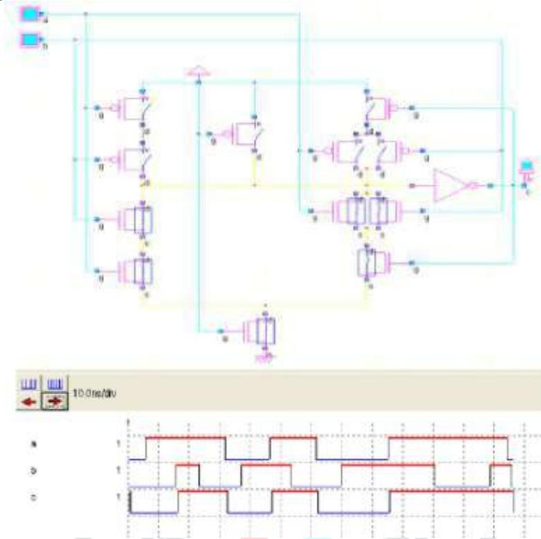
Design and Simulation of Proposed Ring Counter of Double edge triggered Flip Flop with Clock Gated by C-Elements
