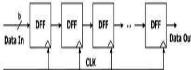
Figure 1 Delay Buffer implemented by Shift Register
