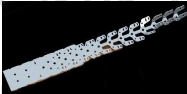
Figure4. Strip Layout for the required component
