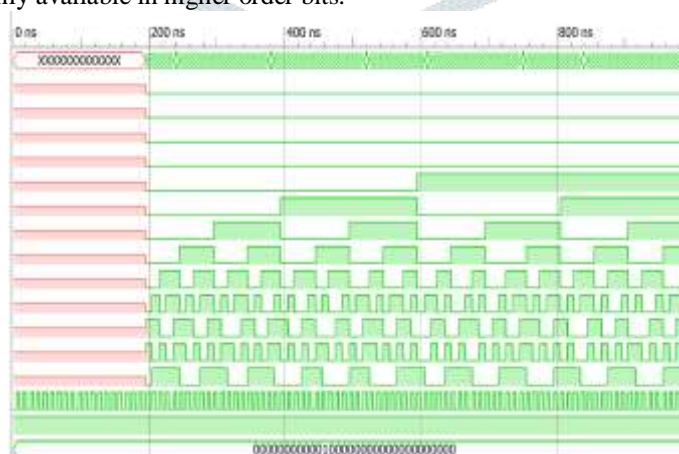
Figure 6 Phase accumulator output for fout = 10MHz
