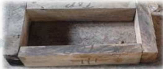
Fig.2: Photograph of Customized Wooden Frame for Making Two Custom Brick Samples
