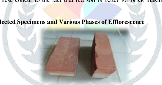
Fig.6: Photograph Showing Selected Pair of First Class Brick with ‘Nil’ efflorescence
