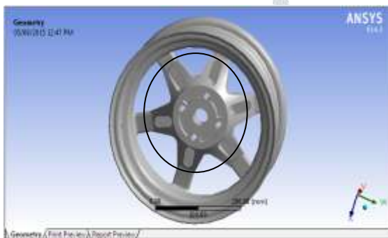
Fig.3.1 3D Model of Optimized Model Wheel
