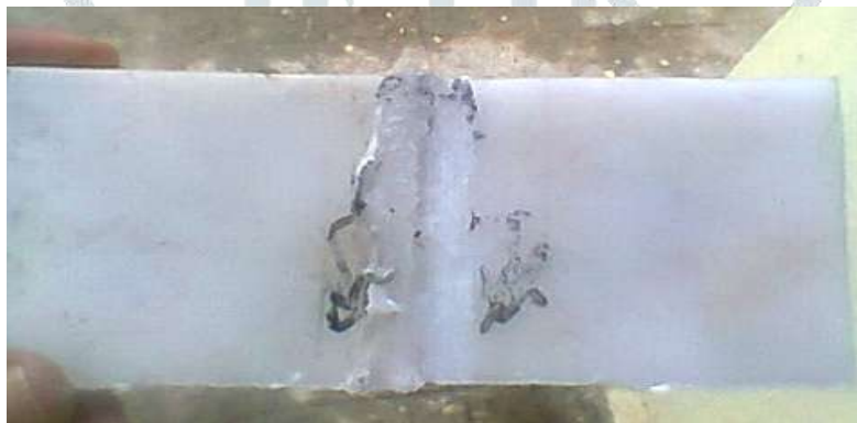
Fig.4. Friction stir welded polyethylene joint.(550rpm and 2.53 Tonnes).
