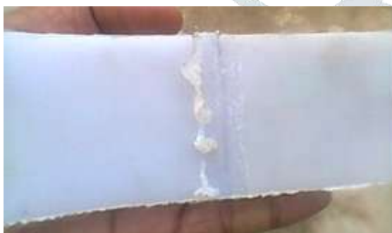
Fig. 5. Friction stir welding of polyethylene (750rpm and 2.68 Tonnes).
