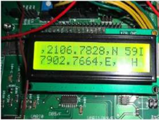
Figure 11: Output of GPS on LCD Screen
