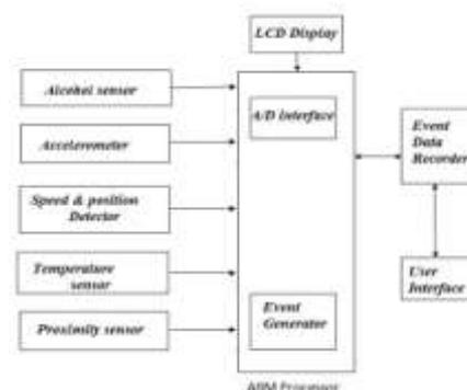
Fig.1 Block diagram of event data recorder
