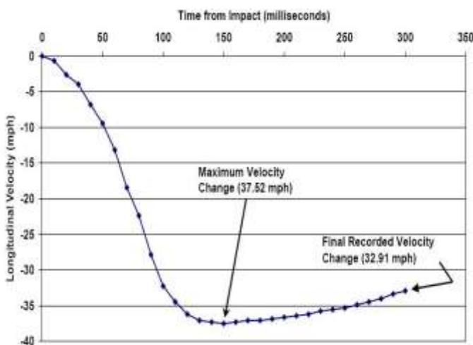
Fig 3: GM EDR record for longitudinal velocity vs. time
