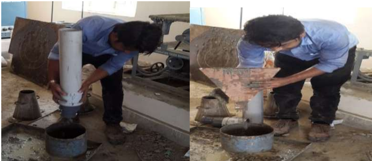
Fig. 4.9: Performing Orimet Test (Flow Time in second) and V-funnel test
