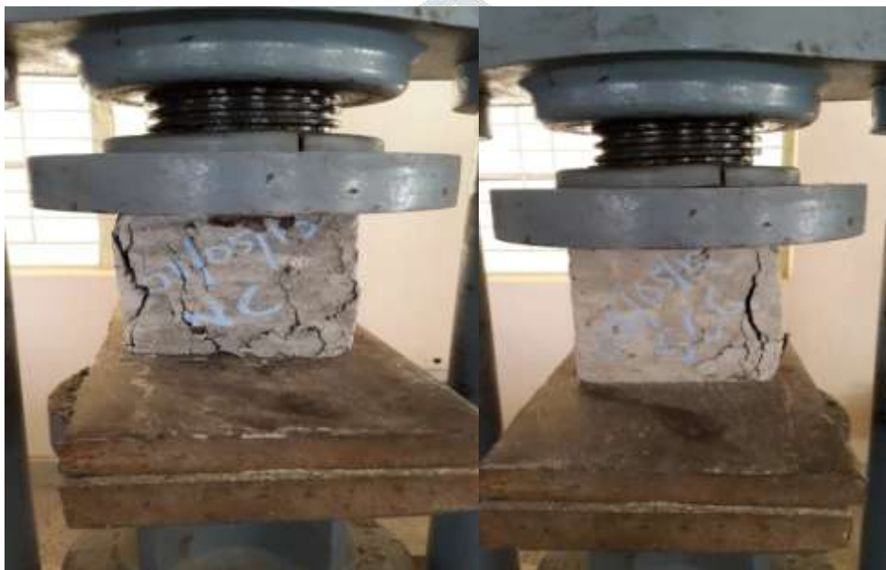
Fig. 4.1: Performing compressive strength test for 28 days
