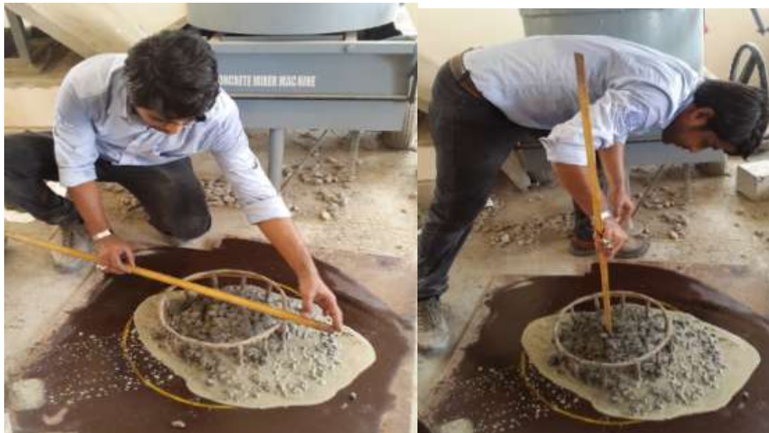
Fig. 4.11: Performing Slump Flow/J-Ring combination test
