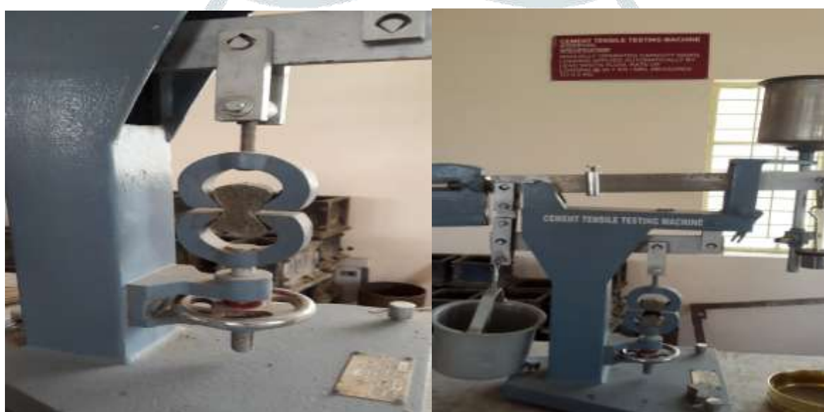
Fig. 4.3: Performing tensile strength test for 7 days
