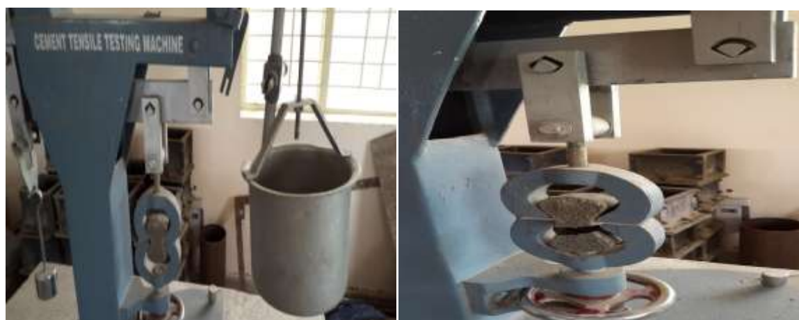
Fig. 4.4: Performing tensile strength test for 28 days
