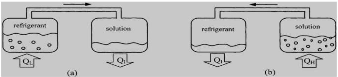
Fig. 1(a): Absorption process occurs in right vessel causing cooling effect in the other;
