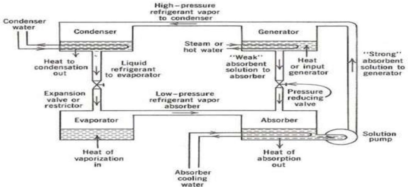
Fig. 1(b): Refrigerant. Fig. 2: Schematic diagram of absorption refrigeration system
