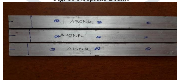
Fig. 11 Natural Rubber Beams
