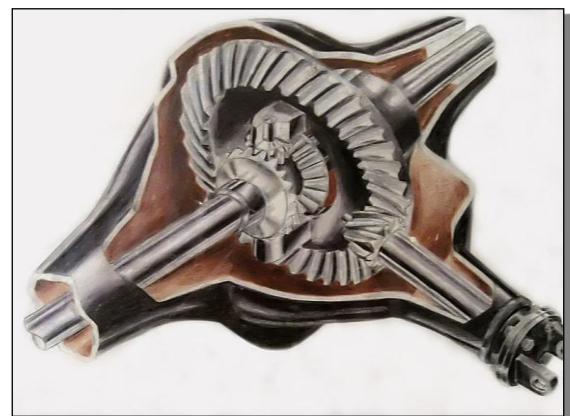
Fig 1.2: Functional description of differential
