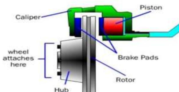
Disc brakes are fairly simple to work with. Typically, there are four main parts of a disc brake system as given below:
