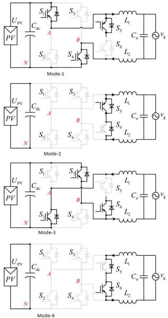
**Fig.4. Conduction Modes of HERIC Topology**
