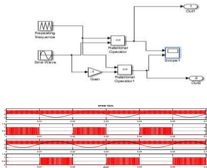
Fig.5. Simulation of SPWM Technique [11]-[12]
