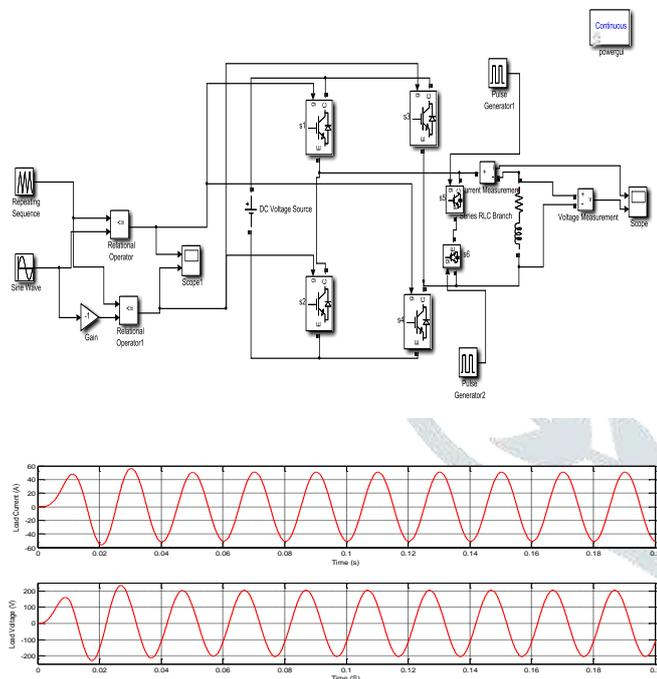
Fig.6. Simulation O/P Result of HERIC Topology
