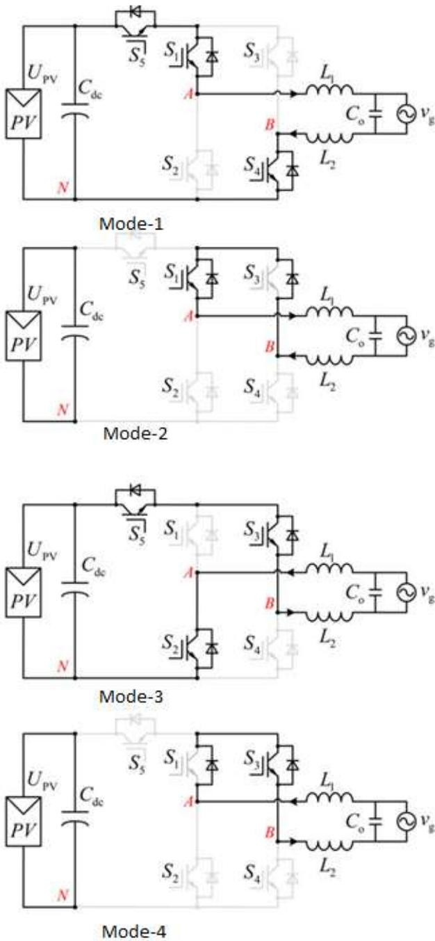
**Fig. 3. Conduction Modes of H5 Topology**
