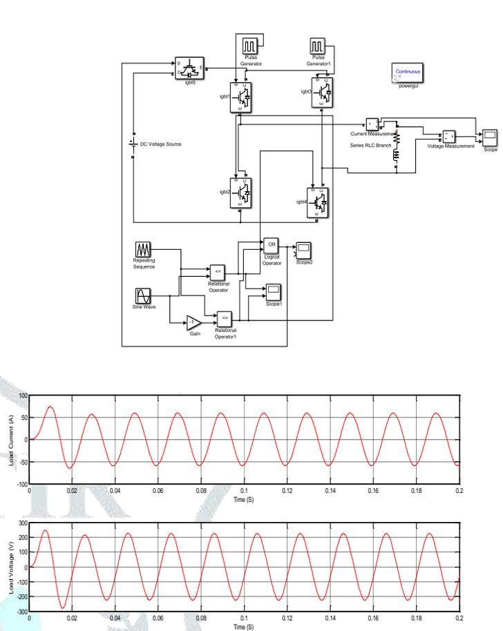
Fig. 7. Simulation & O/P Result of H5 Topology
