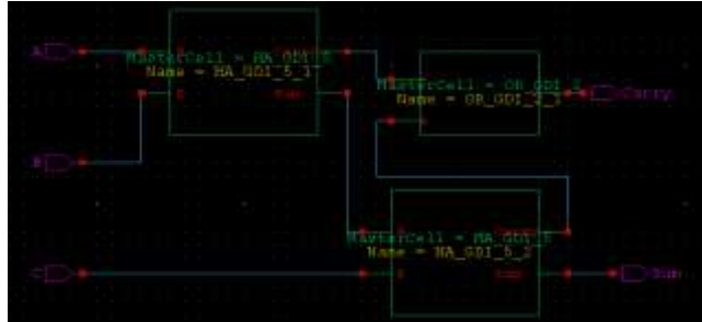
Fig.6 1-BIT FULL ADDER BY GDI
