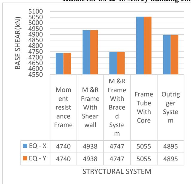
Fig. 12 Base shear for 30 storey model
