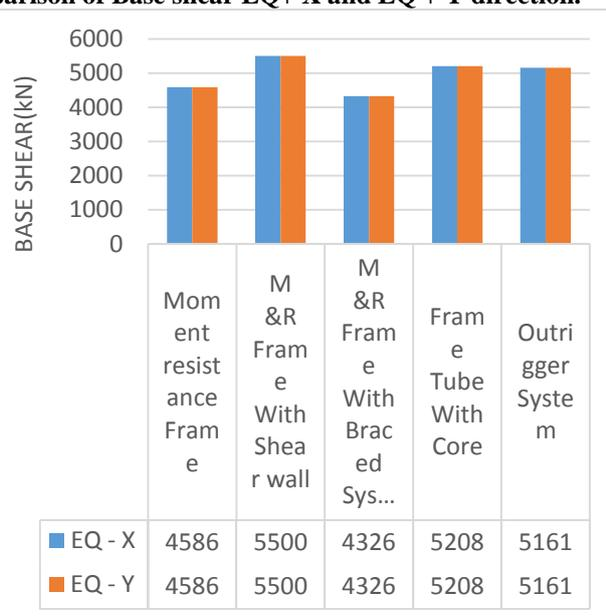
Fig. 13 Base shear for 40 storey model
