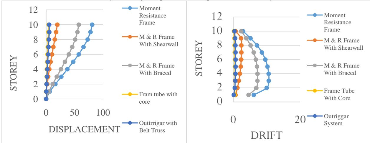
**Fig. 2 displacement for 10 storey model**
