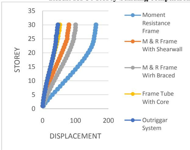
**Fig. 6 displacement for 30 storey model**
