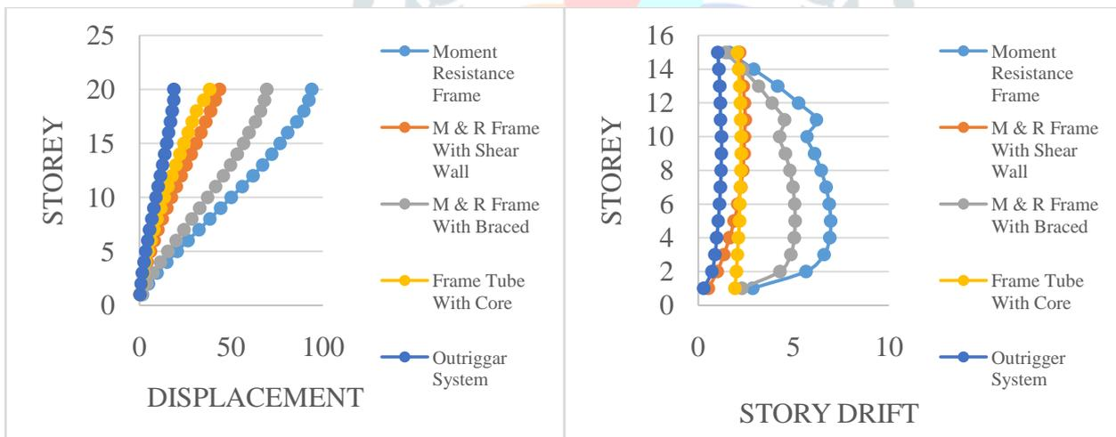
**Fig. 4 displacement for 20 storey model**
