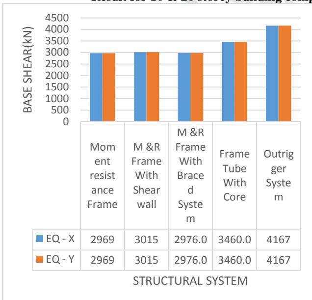
**Fig. 10 Base shear for 10 storey model**
