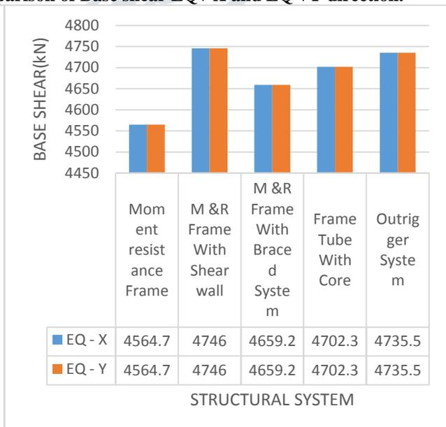
**Fig. 11 Base shear for 20 storey model**
