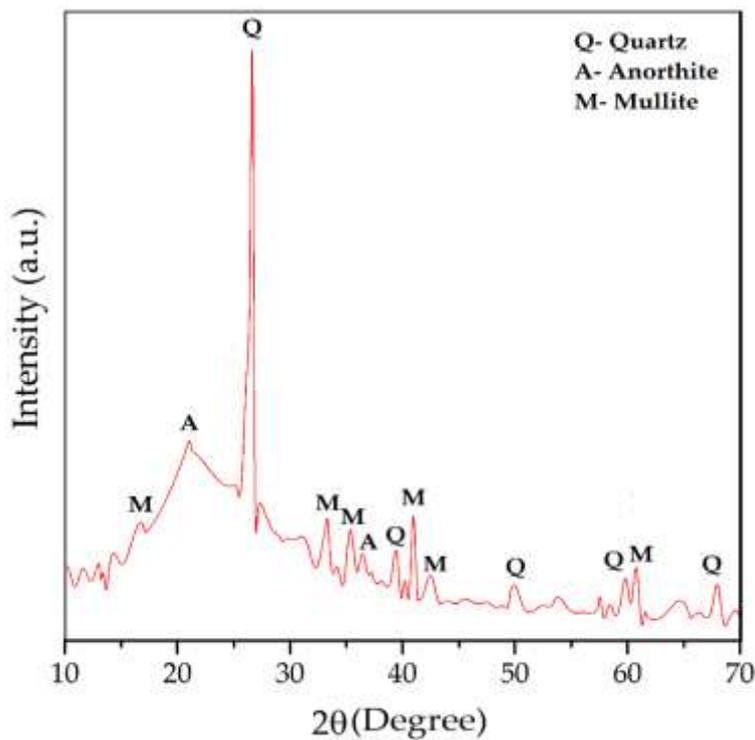
Fig 5: X-Ray Diffraction pattern for sample 5G6R
