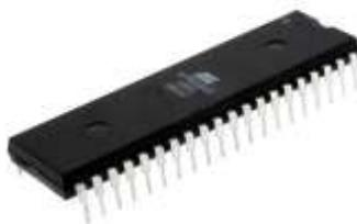
A microcontroller is a single chip that contains the processor (the CPU), non-volatile memory for the program (ROM or flash), volatile memory for input and output (RAM), a clock and an I/O control unit.
