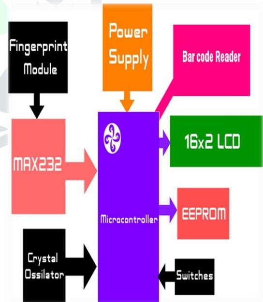
Stamping facility which enables them to record the exact time and date whenever a key is pressed. On completion of Barcode and finger print verification, the voting module powers on and the person can cast his vote by simply pressing the button corresponding to the name of the desired candidate.
