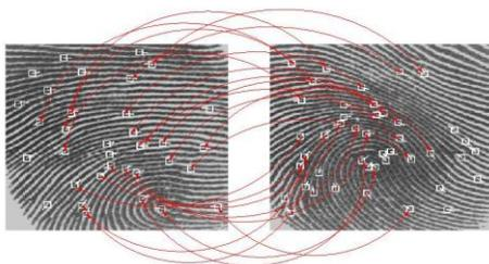
If the processor finds that the image is crisp and properly exposed, it proceeds to comparing the captured fingerprint with fingerprints on file. If the finger print matches, a signal will be sent to the programmed microcontroller.
