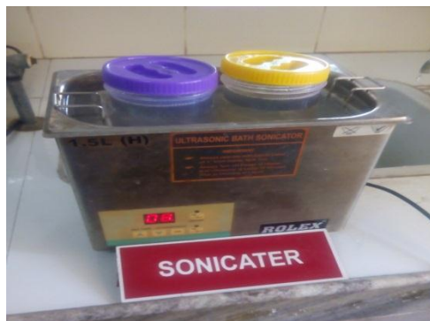
Fig. 7 Nano lubricant on Ultrasonic vibrator
