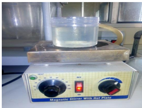
Fig.6 Nano lubricant on magnetic stirrer
