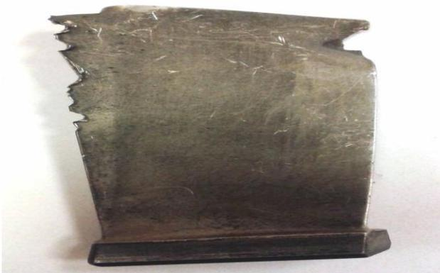
Figure 1: View of blade damaged
