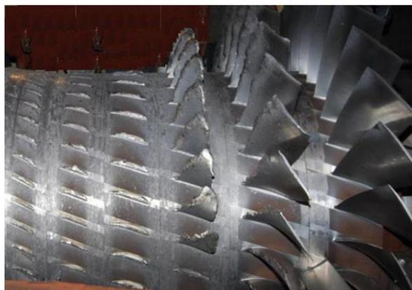
Fig. 1. Photograph of failed compressor rotor.
