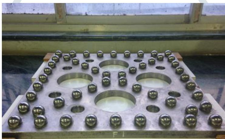
Figure 3 CMM Calibration plate (measured)
