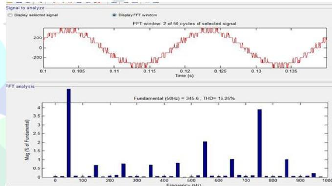
Fig.4 Harmonic Spectrum of Five level diode clamped Inverter Phase Voltage at modulation Index=1 (PD PWM Technique)
