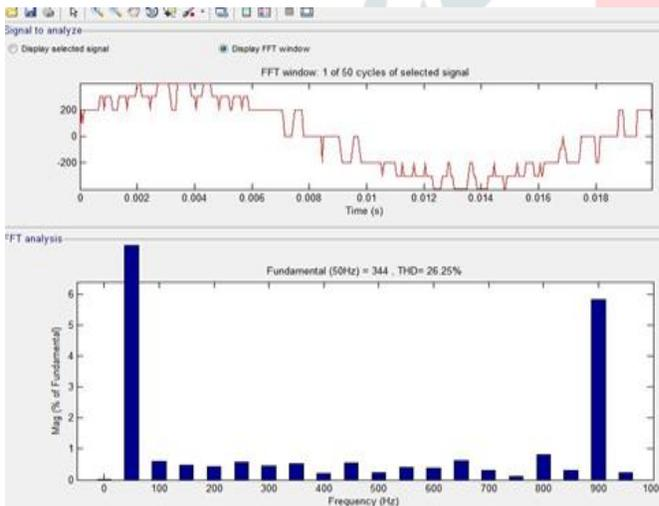
Fig.12 Harmonic Spectrum of Five level diode clamped Inverter Phase Voltage at modulation Index=1 (APOD PWM Technique).
