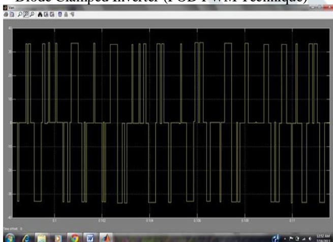
Fig.7 CMV of Five Level Diode Clamped Inverter(POD PWM Technique)
