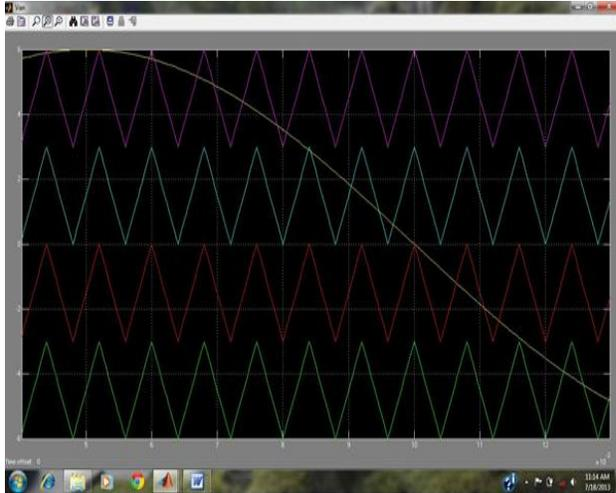
Fig. 1 Sine Waveform Simulation of Five Level Diode Clamped Inverter.(PD PWM Technique)
