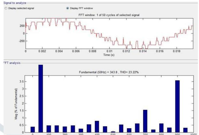
Fig.8 Harmonic Spectrum of Five level diode clamped Inverter Phase Voltage at modulation Index=1 (POD PWM Technique)
