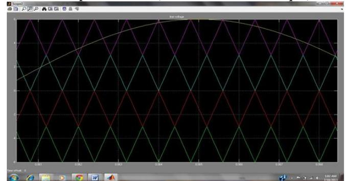
Fig 10 Triangular Waveform Simulation of Five Level Diode Clamped Inverter (APOD PWM Technique)
