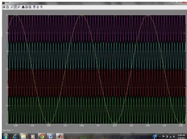
Fig.5 Sine Waveform Simulation of Five Level Diode Clamped Inverter.(POD PWM Technique)
