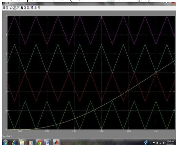
Fig.6 Triangular Waveform Simulation of Five Level Diode Clamped Inverter (POD PWM Technique)
