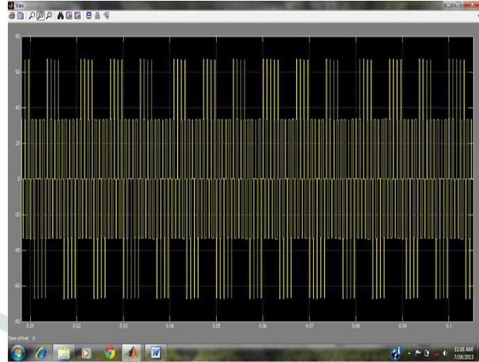
Fig. 3 CMV of Five Level Diode Clamped Inverter(PD PWM Technique)
