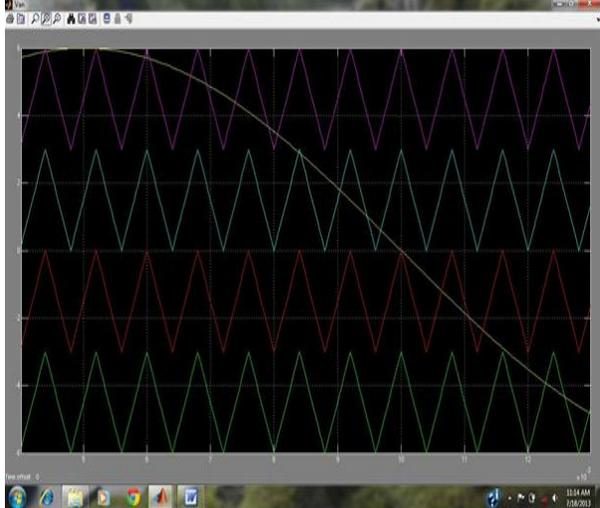
Fig.2 Triangular Waveform Simulation of Five Level Diode Clamped Inverter (PD PWM Technique)
