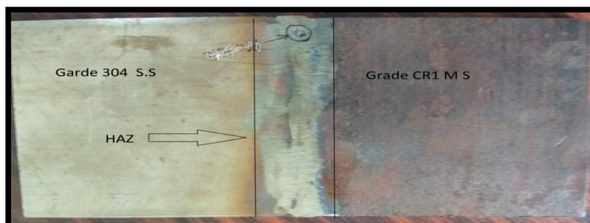
**Figure: 3. TIG welded Plates.**
