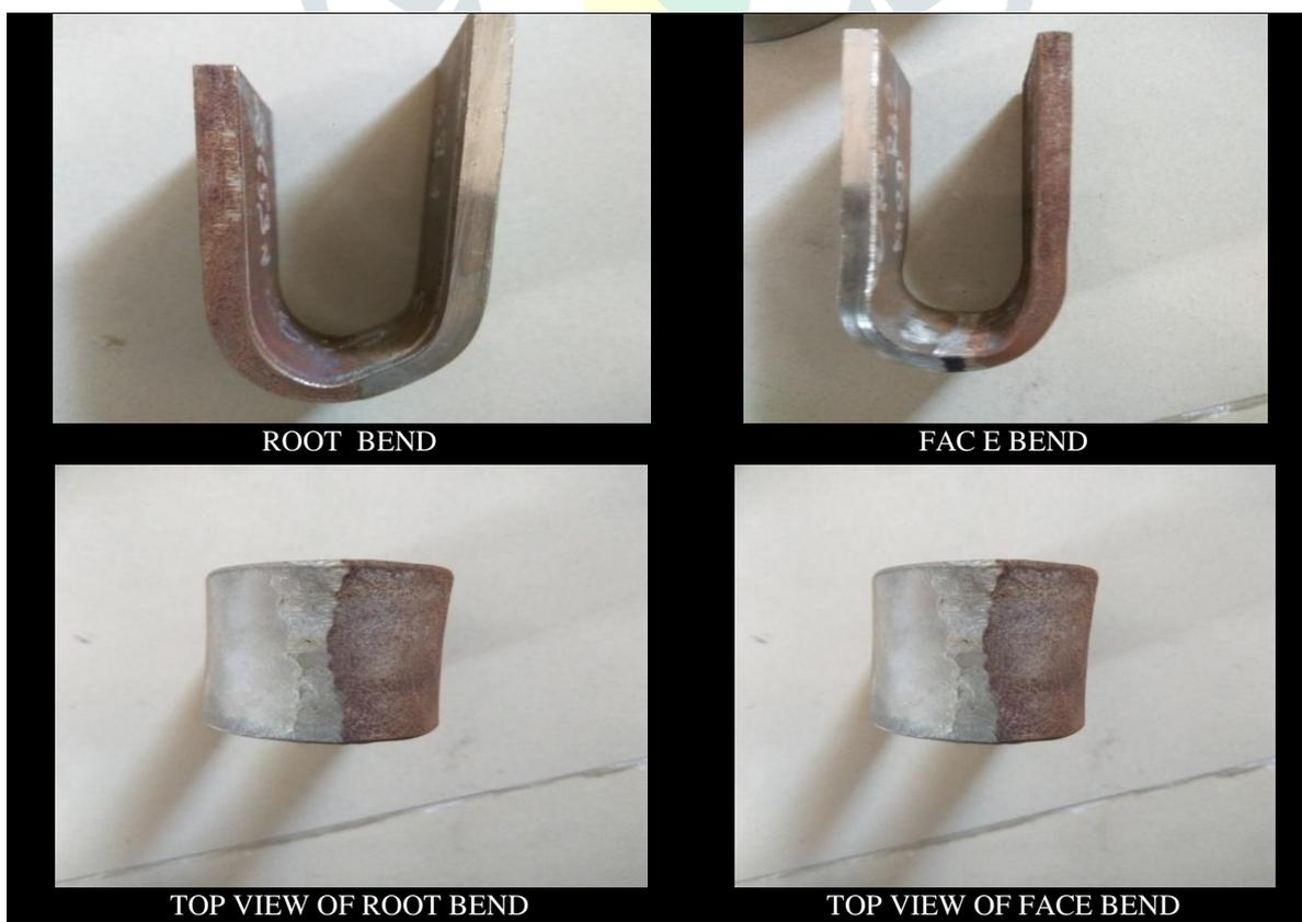
**Figure: 11. Bend tested Specimen**
