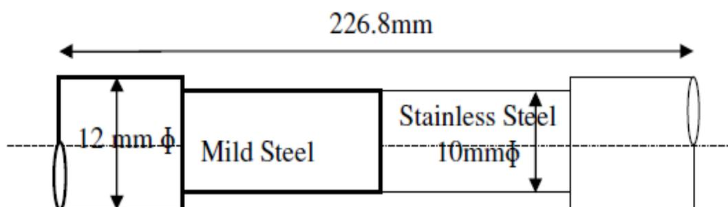
Figure: 8. Standard Tensile specimen
