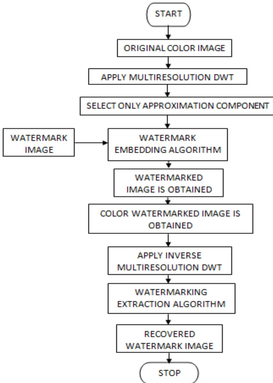
FIGURE 2: FLOW CHART OF PROPOSED WATERMARKING ALGORITHM
