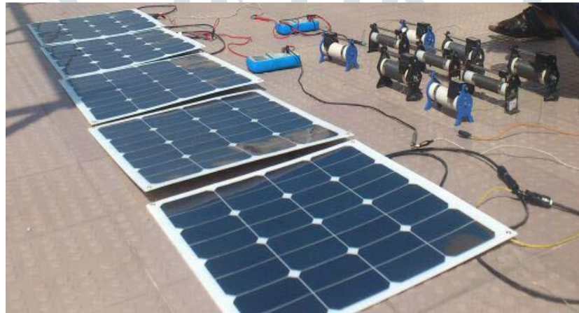
FIGURE 4: THE 50 W SEMI-FLEXIBLE SOLAR PANELS USED FOR THE ASSEMBLY OF ENVIRONMENTAL FRIENDLY CAR.
