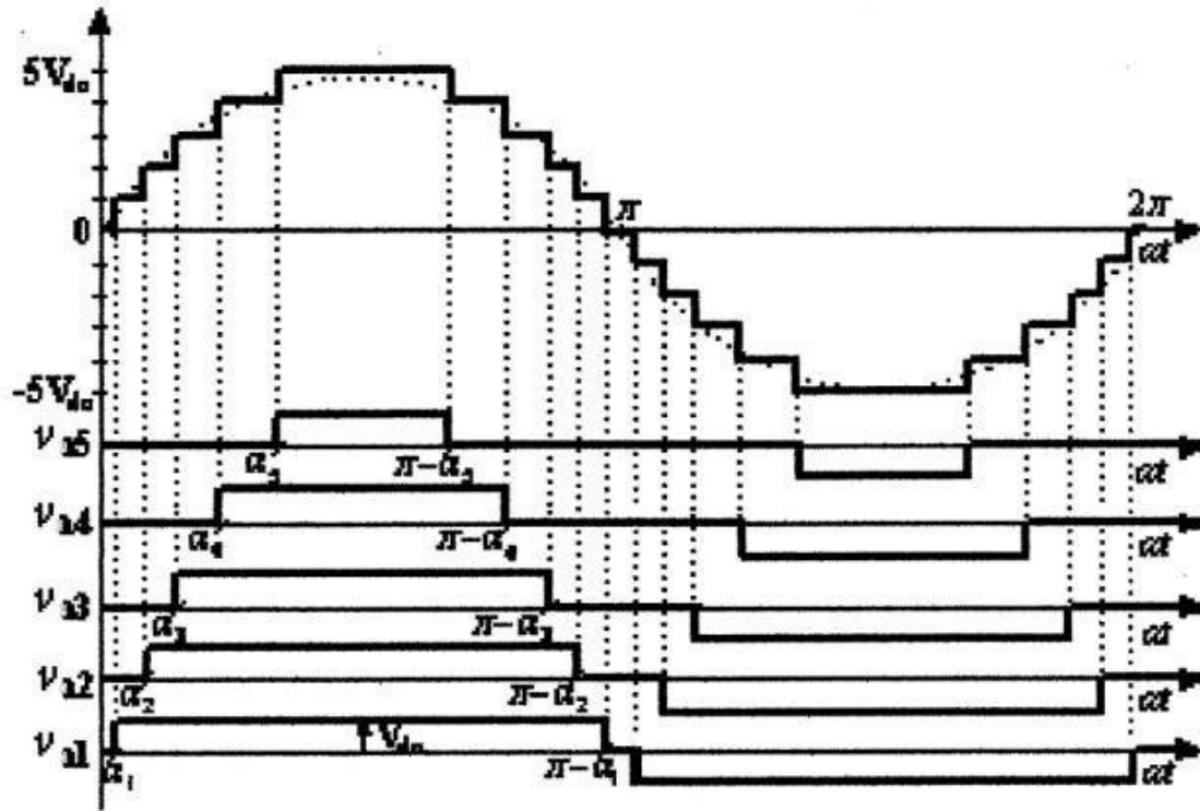
Fig.3. Diagram of output-voltage phasors at switching frequency for the 11-level H-bridge cascaded inverter
