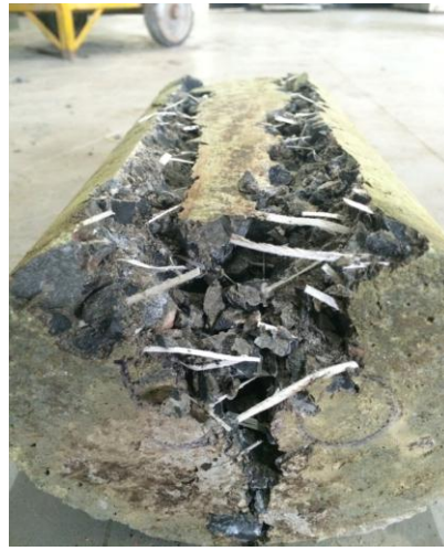
Figure 2: Ductile behavior of concrete cylinder with PP fibers
