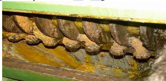
Fig. 1: Screw press without barrel cage to show worm sections
