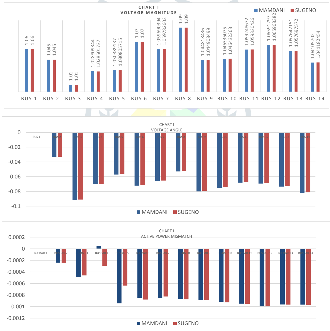
CHART I FUZZY LOAD FLOW SOLUTION FOR "14-BUS" TYPICAL TEST SYSTEM POWER MISMATCHES (ACTIVE / REACTIVE) = 0.001 p.u.
