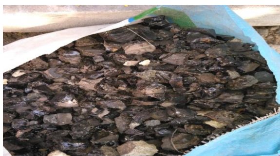
Fig -2: 20mm sized of Cupola Slag aggregate (Source: Image Capture)
