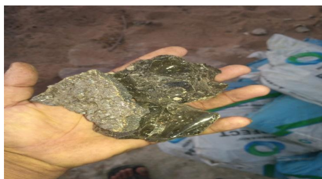
Fig -1: Lump sized of Cupola Slag aggregate (Source: Image Capture)
