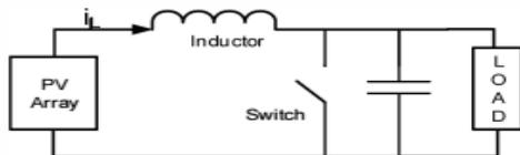
Fig. 6: PV Array Connected Boost Converter
