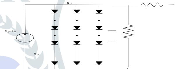
Fig 2: Equivalent Circuit of a number of solar cells in series & parallel
