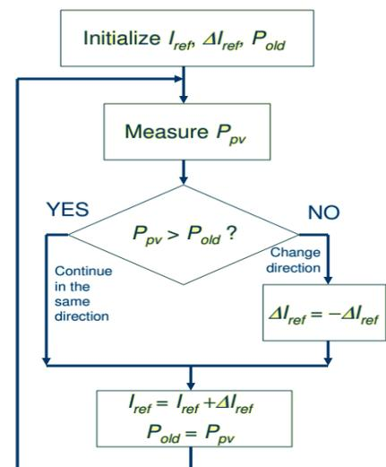
Fig. 8: "Perturb & Observe" MPP Tracking Algorithm
