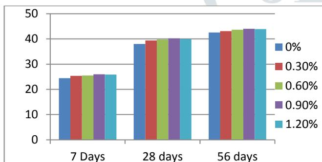
**Chart 1** compressive strength of nominal concrete and steel fiber concrete
