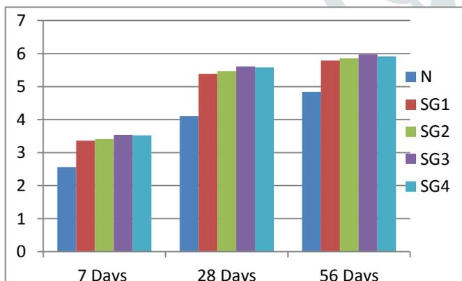
**Chart 6** Flexural strength of steel and glass fiber concrete
