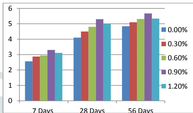
**Chart 3** Flexural strength of nominal concrete and steel fiber concrete
