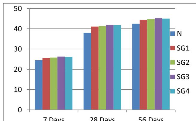
**Chart 4** compressive strength of nominal concrete to steel and glass fiber concrete
