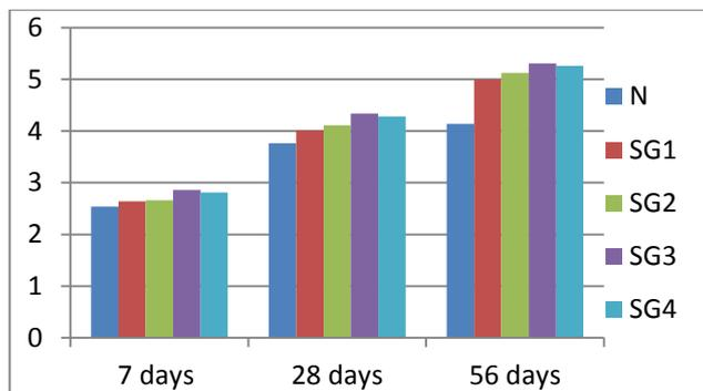
**Chart 5** Split tensile strength of nominal concrete to steel and glass fiber concrete
