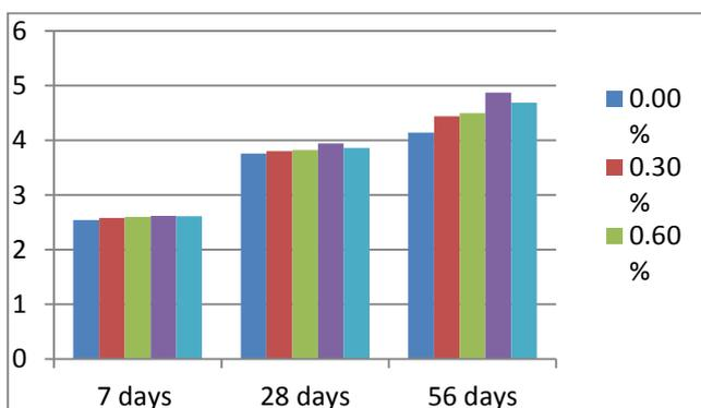
**Chart 2** Split tensile strength of nominal concrete and steel fiber concrete
