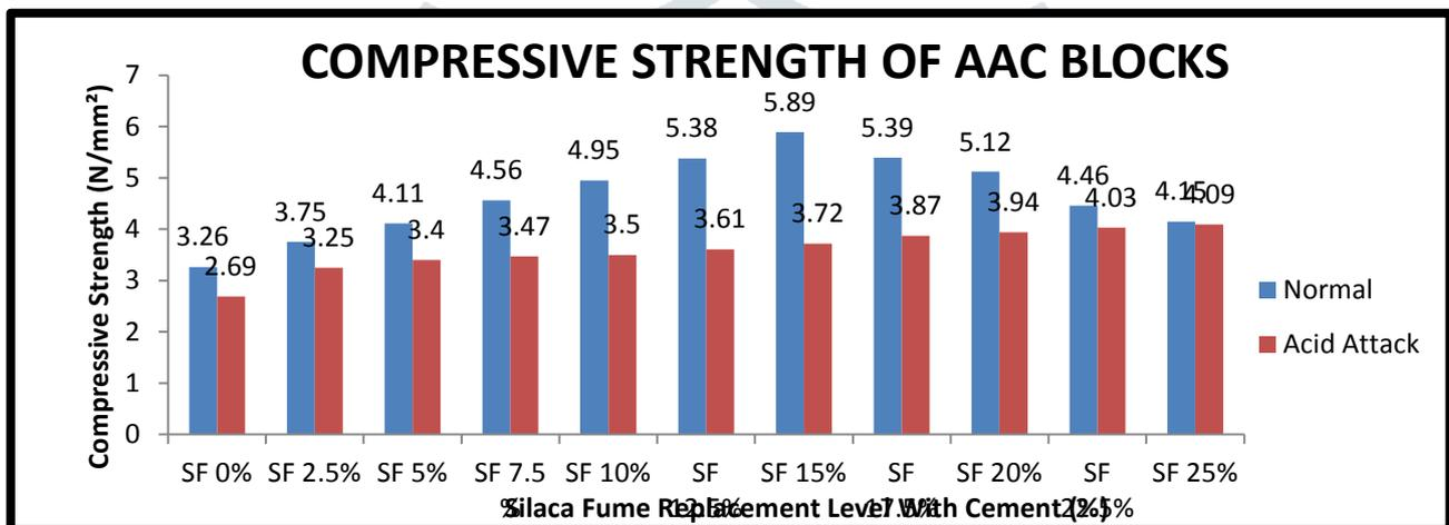
Fig. 1.5(g) Acid Attack of AAC blocks
