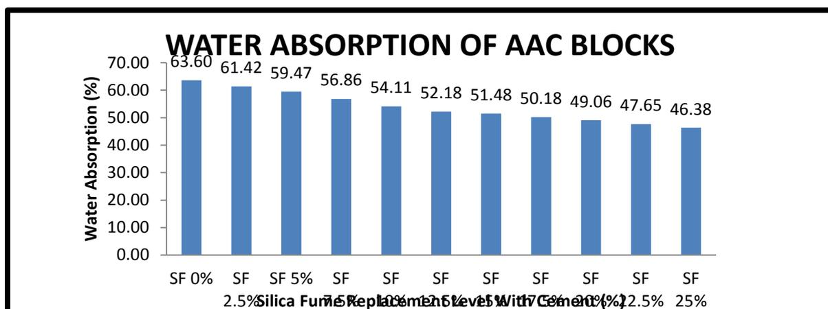
**Fig. 1.5(c) Water Absorption of AAC blocks**
