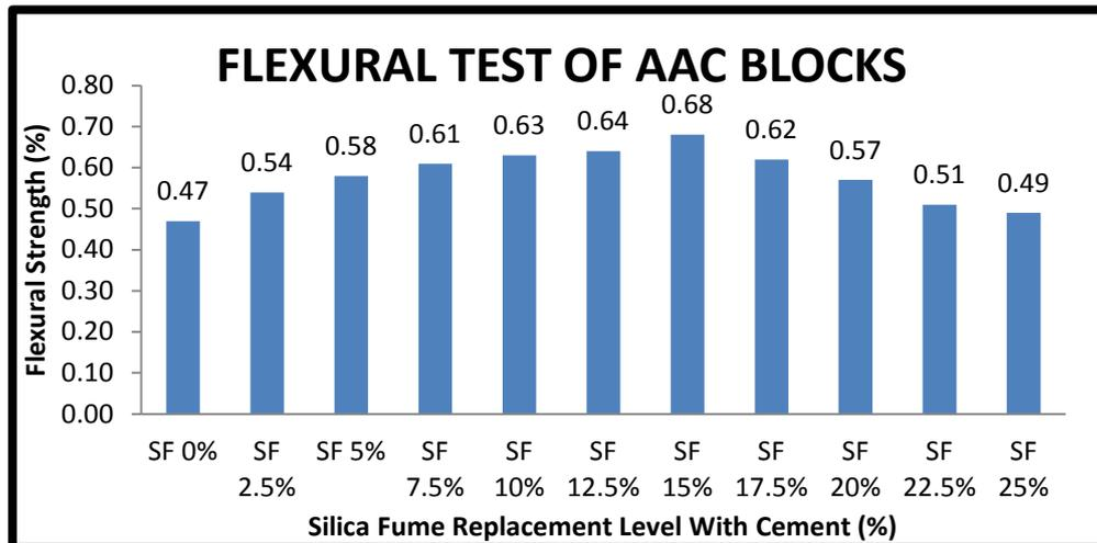
**Fig. 1.5(b) Flexural Strength of AAC blocks**
