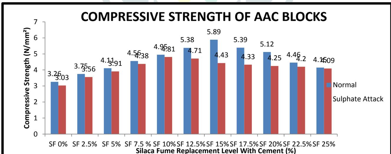
Fig. 1.5(h) Sulphate Attack of AAC blocks
