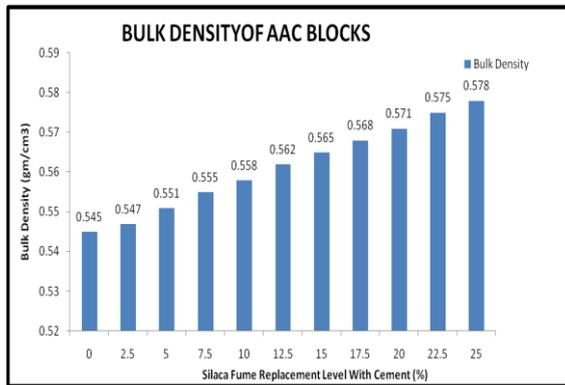
**Fig. 1.5(d<sub>1</sub>) Bulk Density of AAC blocks**
