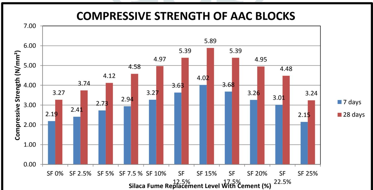
Fig. 1.5(a) Compressive Strength of AAC blocks
