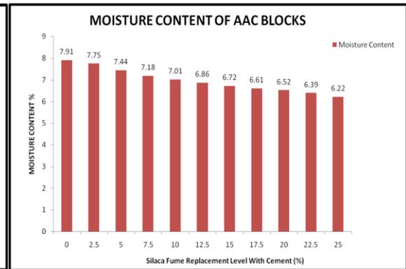
**Fig. 1.5(d<sub>2</sub>) Moisture Content of AAC blocks**
