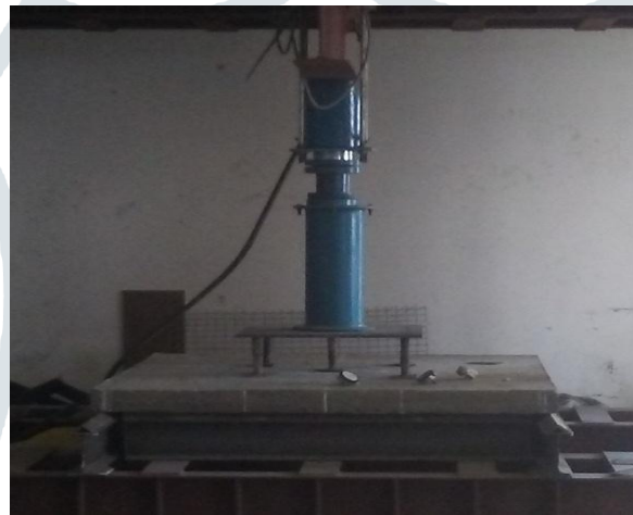
Fig.-2 Slab specimen with five point loading system
