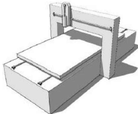
**Figure 3 Moving Table Router**
