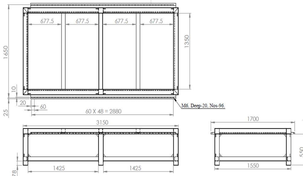
**Figure 5 Detail view drawing CNC Router Structure**
