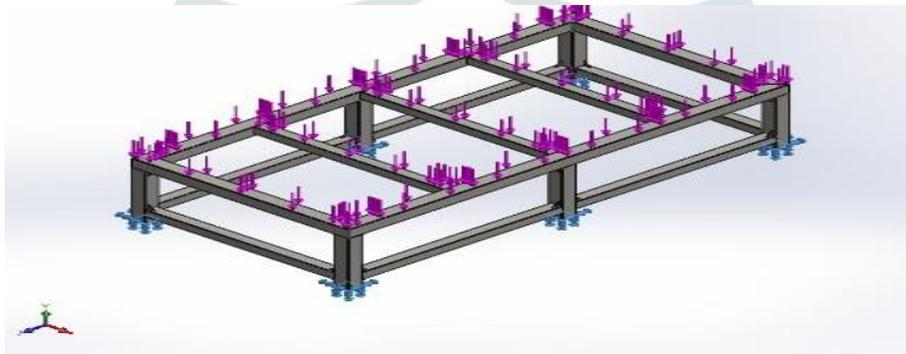
**Figure 8 Boundary condition of NR-115 Base Structure using static analysis**
