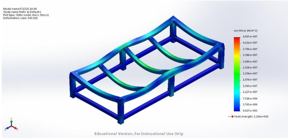
Figure 10 Equivalent Stress analysis of NR-115 Base Structure
