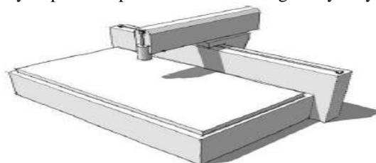
Figure 2 Cantilevered Arm Router
