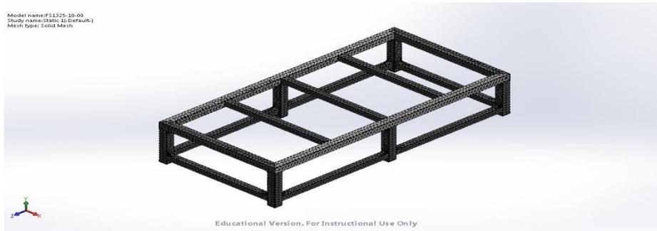
**Figure 7 Meshing of NR-115 Base Structure using static analysis**
