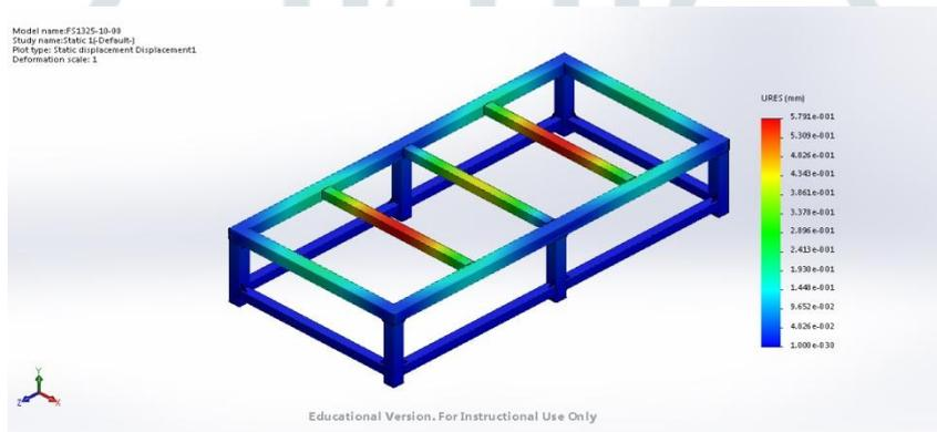
Figure 11 Dis placement of NR-115 Base Structure
