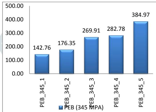
FIGURE 3: MAIN FRAME WEIGHT OF PEB-345 MODELS.
