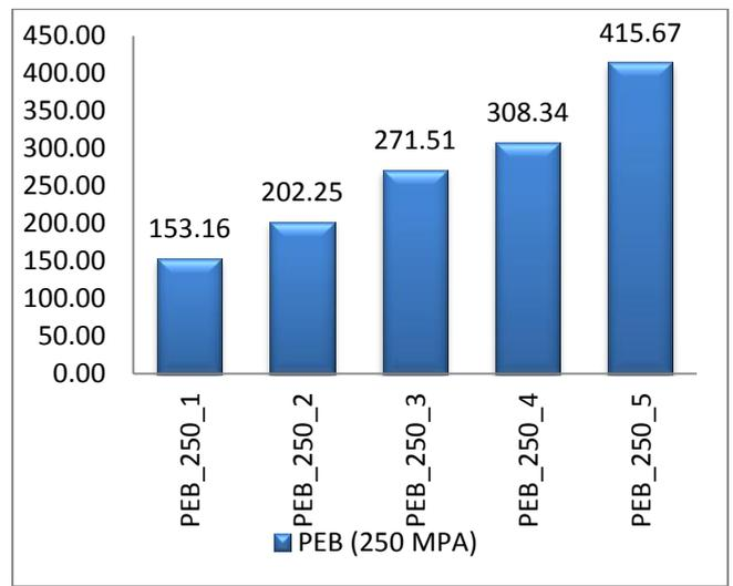
FIGURE 2: MAIN FRAME WEIGHT OF PEB-250 MODELS.
