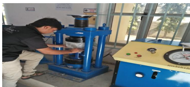
Fig -5: Compression Testing
