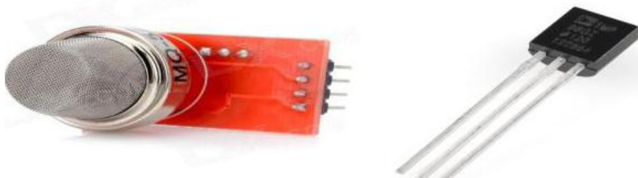
Fig -8: Modules of Gas detector and Temperature sensor
