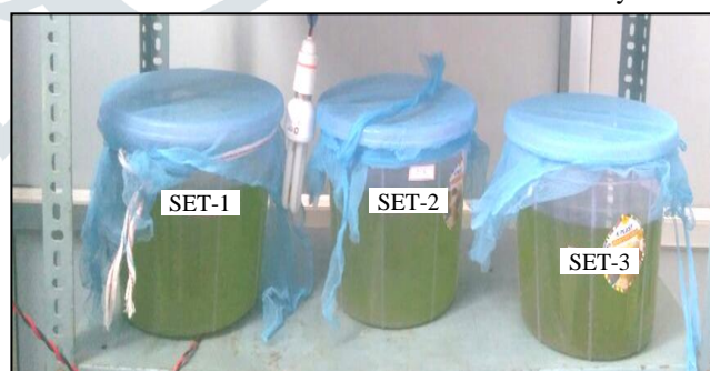
Figure 2: Experimental setup of phycoremediation of tannery effluent in algal consortium
