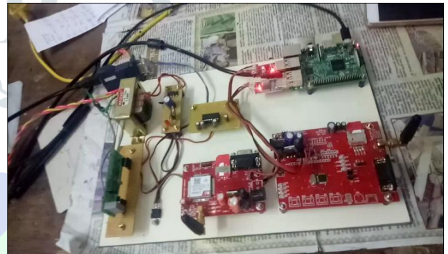
Fig.5: PLC with Raspberry module for IoT communication
