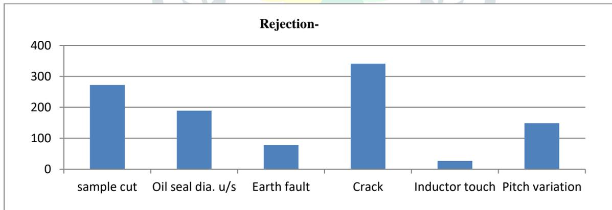
From above graph it has been seen that amount of rejection due to cracks is very high as compare to other causes so it is very important to concentrate on such a factor. So we are selecting crack for analyze to improve the productivity.
