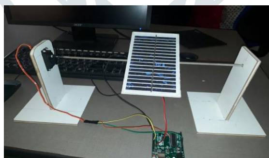
Fig. 14: Solar Tracker setup
