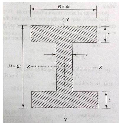
Fig 2: I Section Standard Dimensions of Connecting Rod
