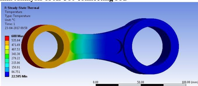
Fig23: Temperature Distribution
