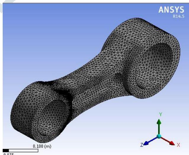
Fig 6: Meshing of Connecting Rod
