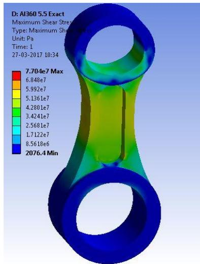
Fig16: Max Shear Stress
