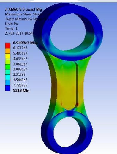
Fig19: Max Shear Stress
