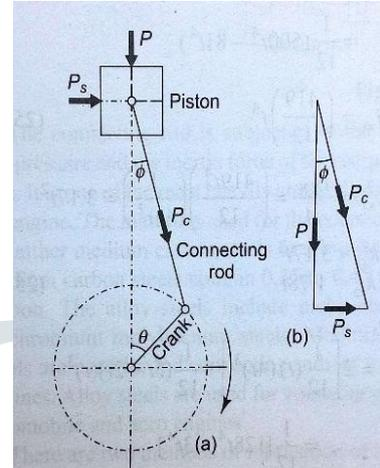
Fig 3: Dead Centre Position for Max Gas Load
