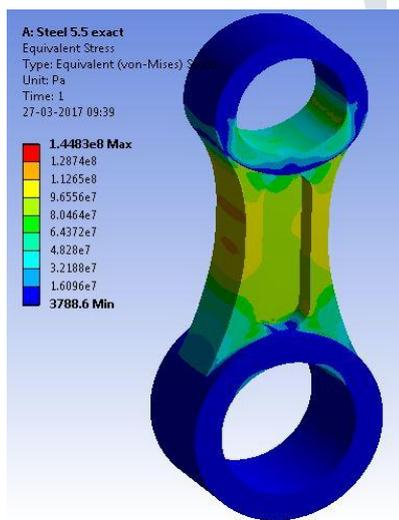
Fig 9: Equivalent Stress
