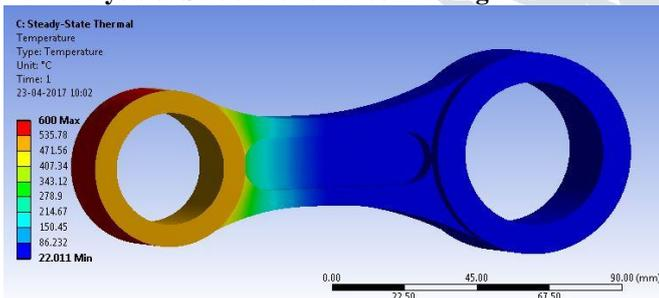
Fig21: Temperature Distribution
