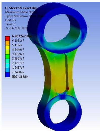
Fig13: Max Shear Stress
