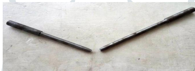
Fig 9. Specimen Breakage under tensile loading
