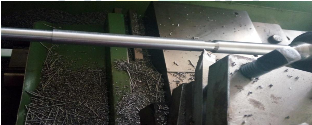
Fig 4. Step turning of M.S Round Bar
