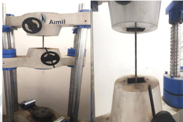
Fig 7 & 8. Specimen holded in U.T.M
