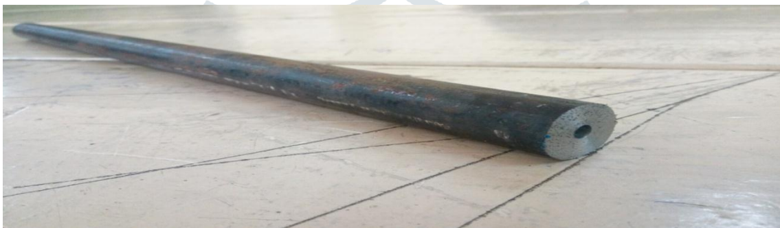
Fig 3. Centre drilling of M.S Round Bar
