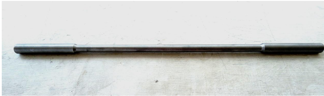
Fig 6. Specimen to test under U.T.M
