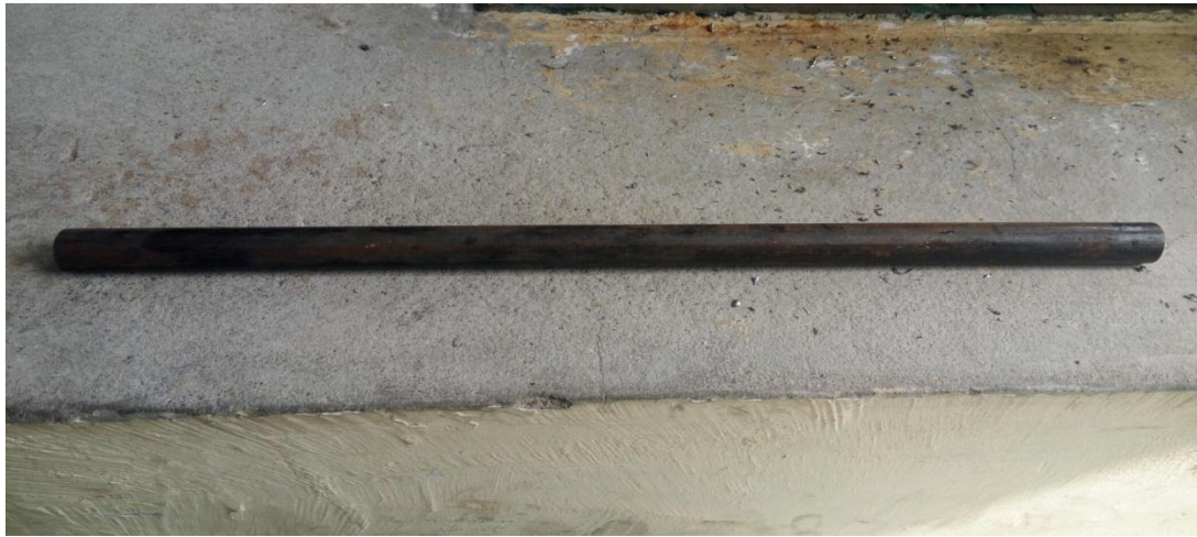
Fig2. Mild Steel Round Bar ( \phi 20×410) mm
