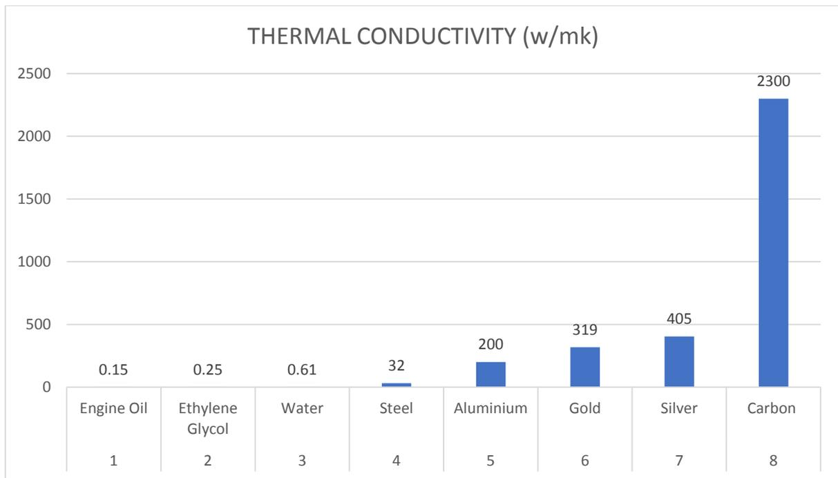
Fig 1- (Thermal conductivities of various material)
