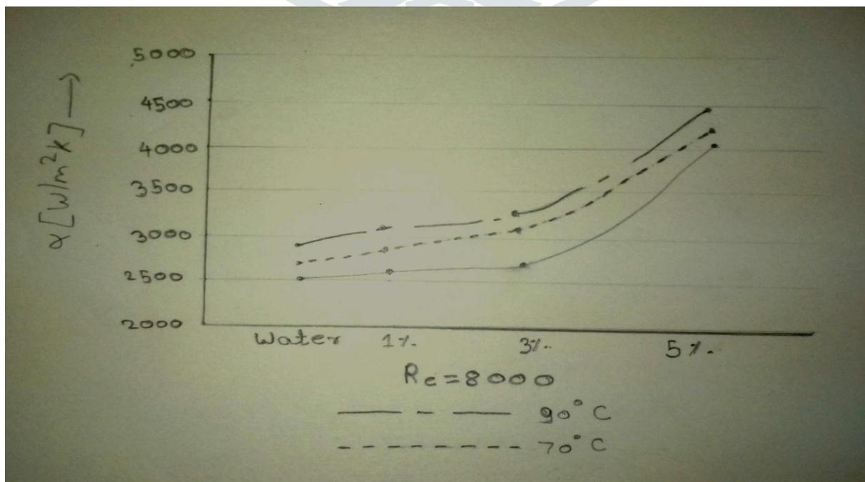
Fig.4 - graph of convective heat coefficients vs nanofluid concentration
