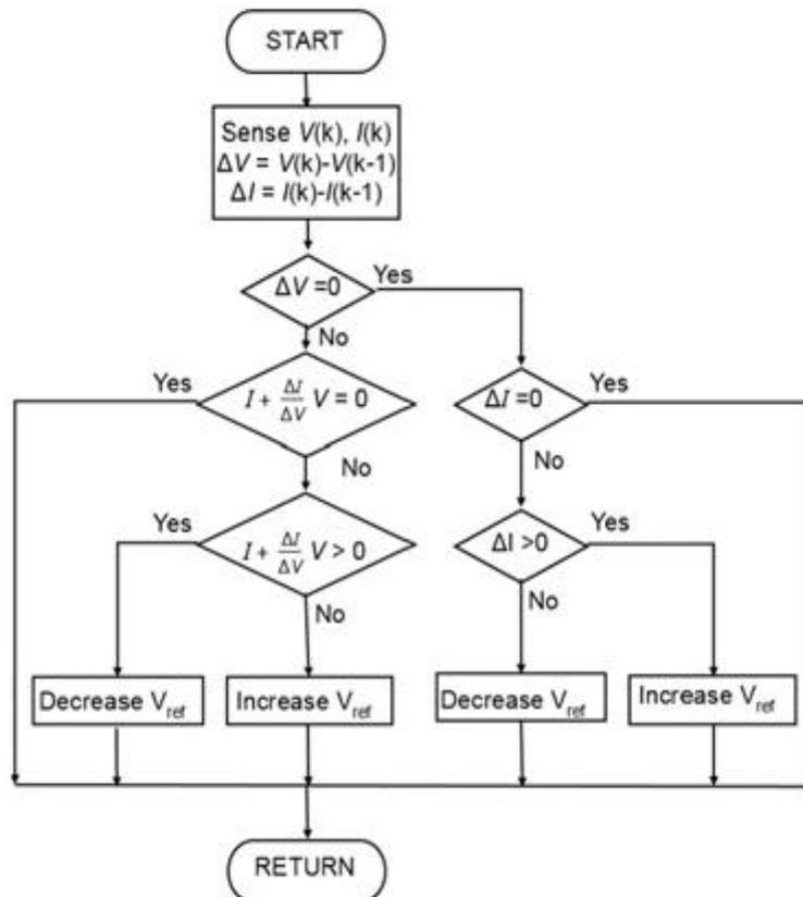
Fig6: Flow chart of MPPT Incremental Conductance Algorithm.
