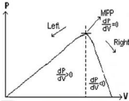
Fig5: Basic Power versus Voltage curve for the MPPT Incremental Conductance Algorithm
