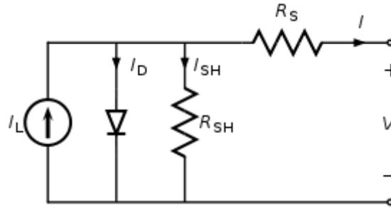
Fig2: Photovoltaic Cell Circuit
