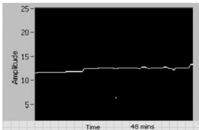
Fig12: Voltage Amplitude Produced from Solar panel with MPPT Incremental Conductance Algorithm.
