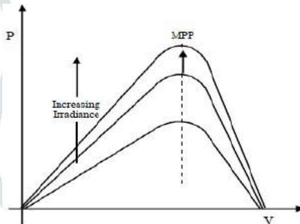
Fig3: Dependence of solar radiation intensity on the output power
