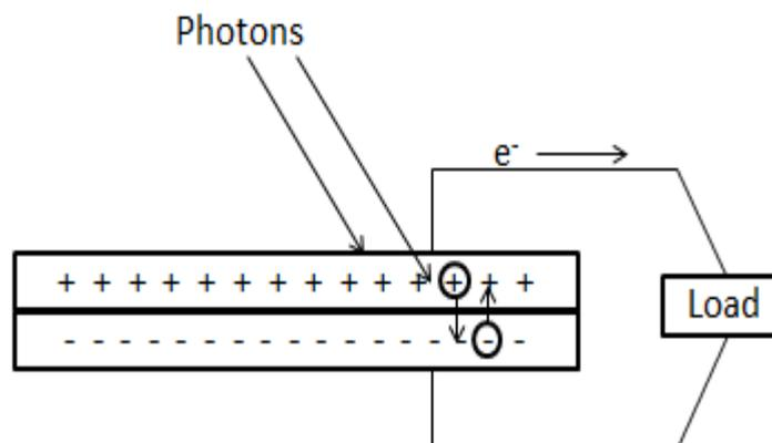
Fig1: PV Cell Working
