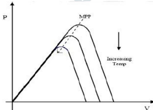
Fig4: Dependence of solar radiation temperature on the output power
