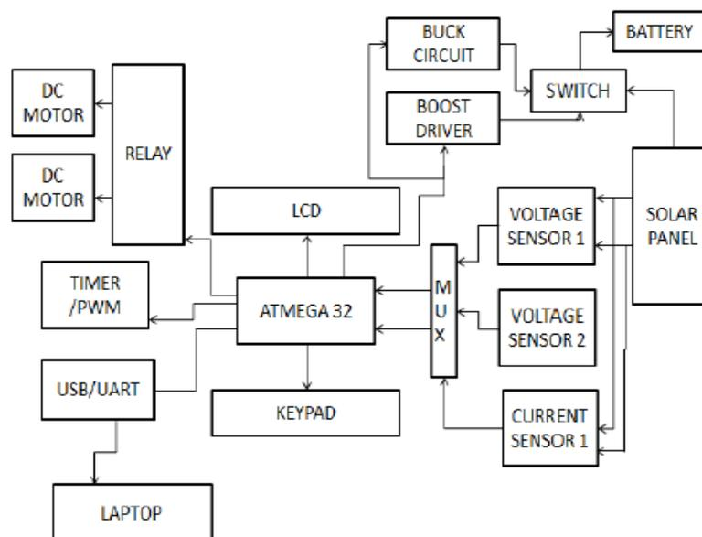
Fig7: Block diagram
