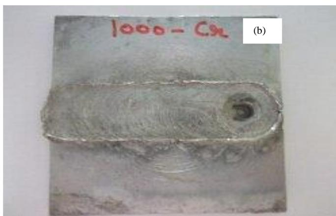
Fig. 2 FSPed plate of (a) Mg/SiC at (1000 rpm), (b) Mg/Cr at (1000 rpm)
