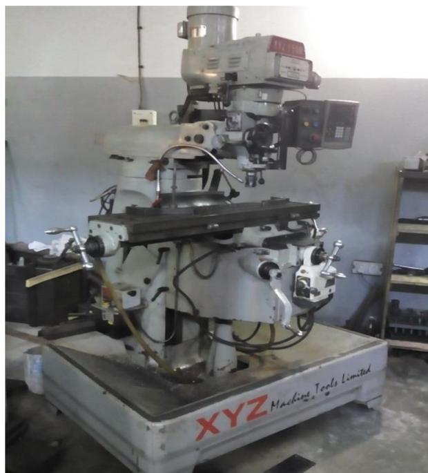
**Fig. 1** Vertical milling machine
