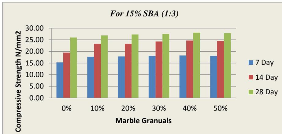
Figure 3: Comp. Strength of Mortar For 1:3 Proportion After Replacement Of 15% SBA
