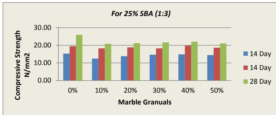
Figure 5: Comp. Strength of Mortar For 1:3 Proportion After Replacement Of 25% SBA
