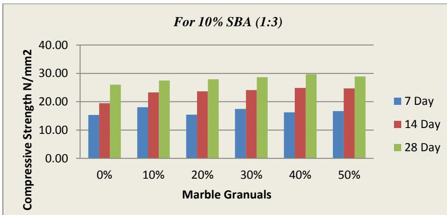
Figure 2. Comp. Strength of Mortar For 1:3 Proportion After Replacement Of 10% SBA
