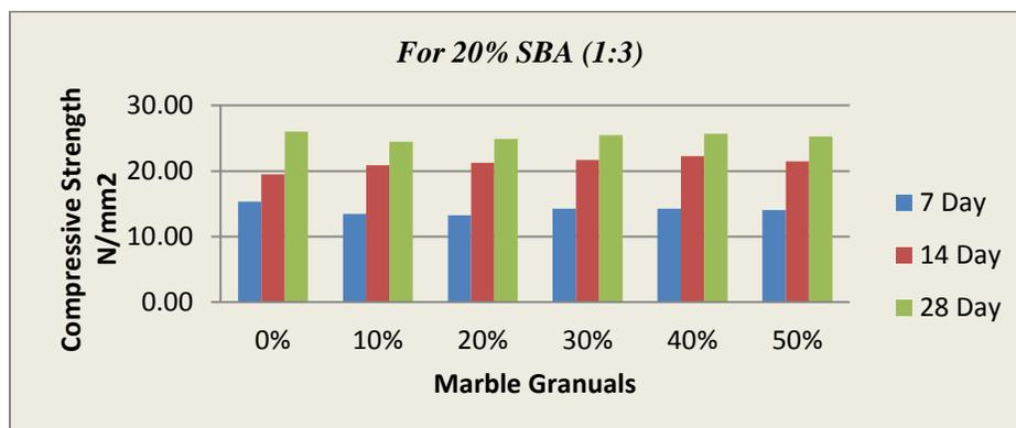
Figure 4: Comp. Strength of Mortar For 1:3 Proportion After Replacement Of 20% SBA
