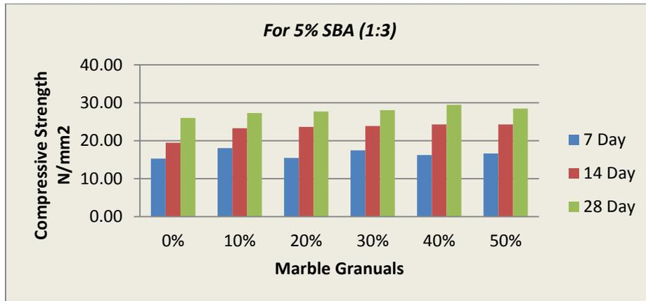
Figure 1 : Comp. Strength of Mortar For 1:3 Proportion After Replacement Of 5% SBA
