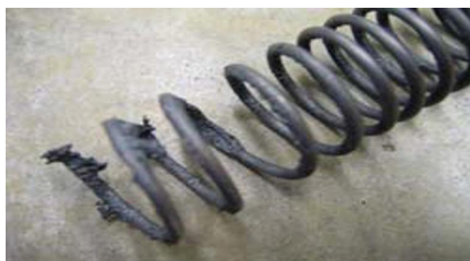
Fig. 5: Photograph of experimental Shchelkin spiral[1].
